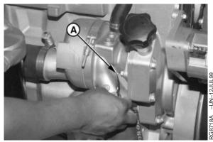
Coolant Pump Weep Hole
