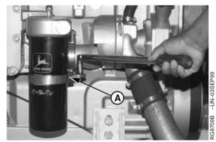
Remove Filter Element Using Wrench
