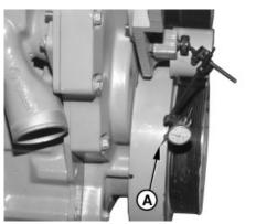
Probe Contacts Damper Outer Diameter
