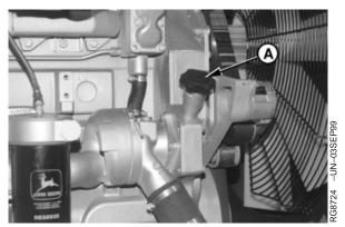
Timing Gear Cover Filler Cap
