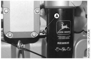
Oil Cooler Housing Drain Valve
