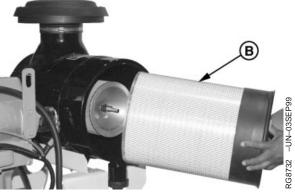
Replacing Primary Air Filter Element
