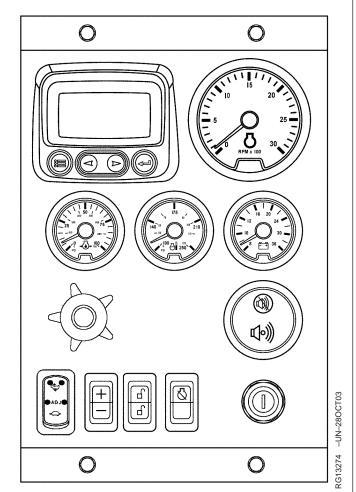
Full-Featured Instrument Panel For Later Engines (See Section 17)
