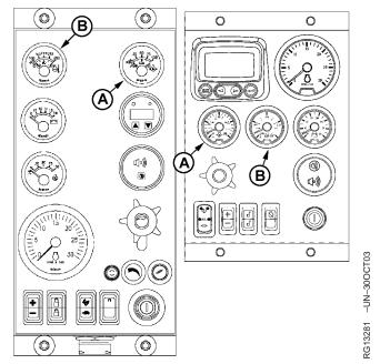
Watch Coolant Temperature and Oil Pressure On Earlier Panel (Left) or Later Panel (Right)
