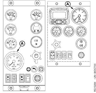
Observe Tachometer Reading On Earlier Panel (Left) or Later Panel (Right)
