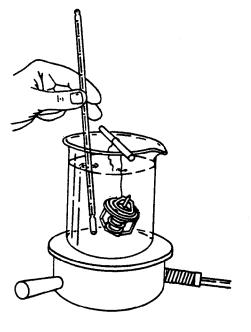
Thermostat and Thermometer in Water
