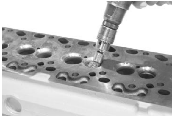
Valve Seat Cleaning and Inspection
