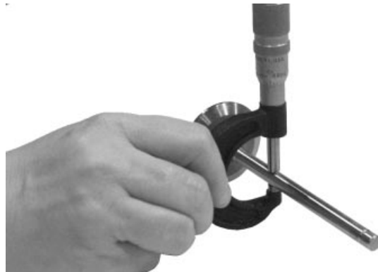
Valve Stem Measurement
