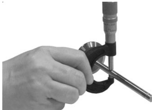
Valve Stem Measurement
