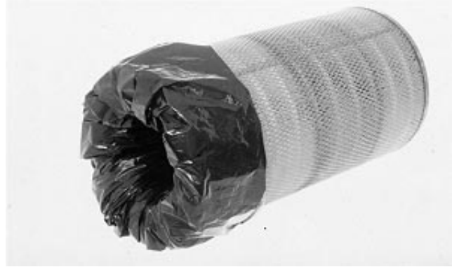
Air Intake Leak Test
