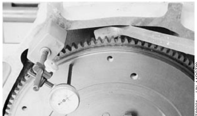
Check Crankshaft End Play w/Dial Indicator
