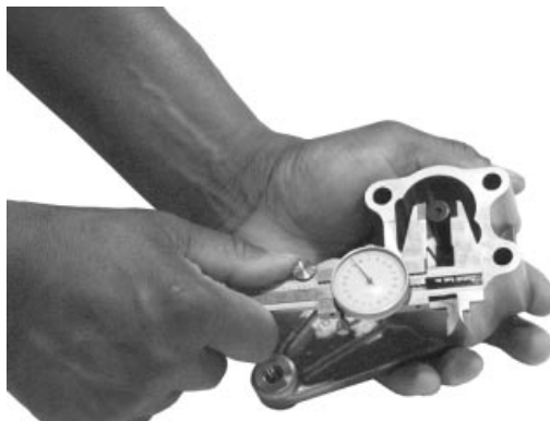
Measure Idler Shaft OD for Wear
