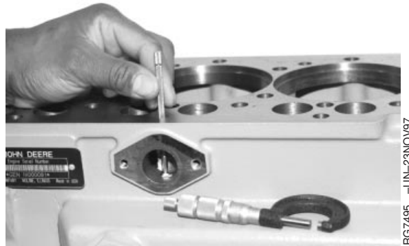
Fuel Supply Pump Push Rod Bore
