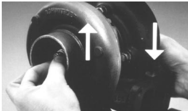
Checking for Contact of Compressor and Turbine Wheels
