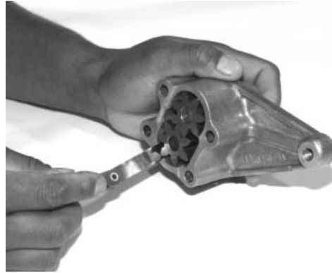
Checking Gear-to-Pump Housing Radial Clearance
