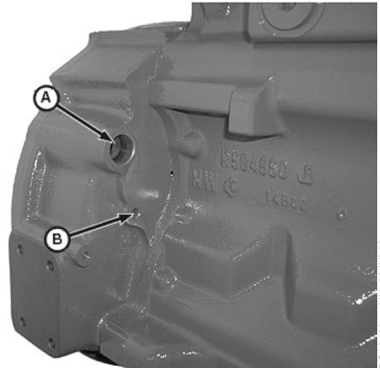
Flywheel Housing Timing Holes
