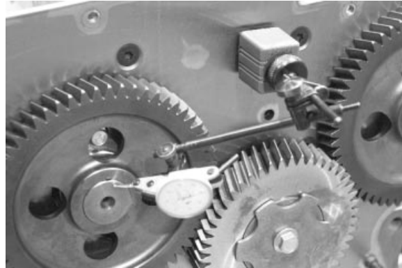
Measuring Camshaft End Play
