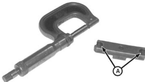
Inspect and Measure Bridges
