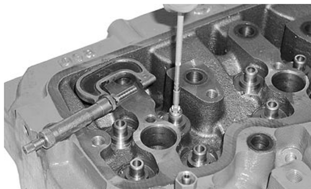
Valve Guide Wear
