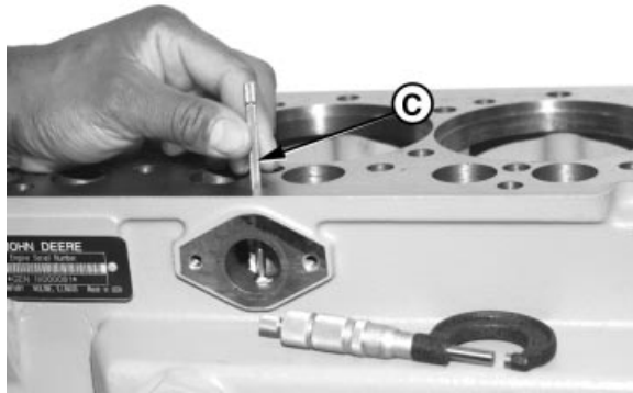
Push Rod Bore in Block Wear
