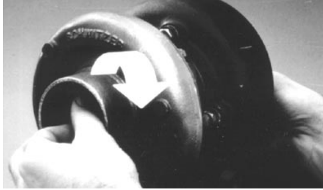
Checking Shaft Rotation and Clearance
