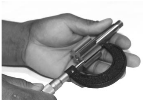
Checking Gear Thickness
