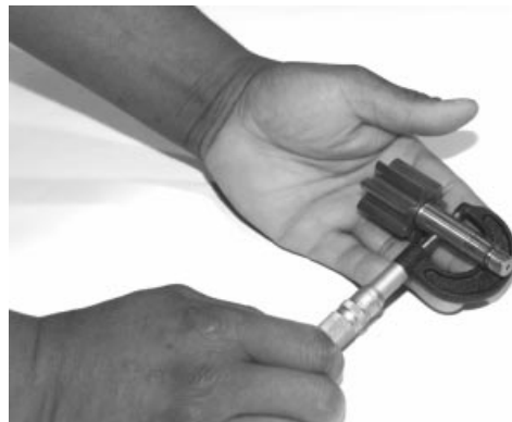
Measuring Drive Shaft OD for Wear
