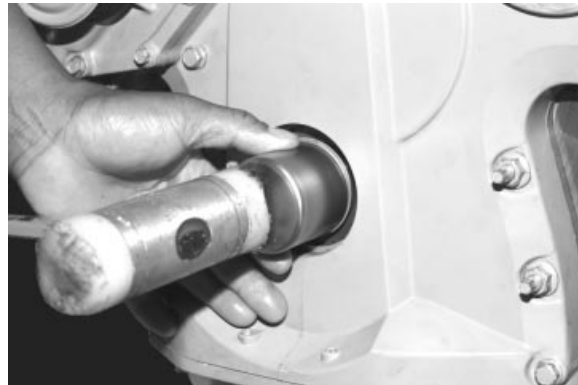
Installing Crankshaft Wear Sleeve
