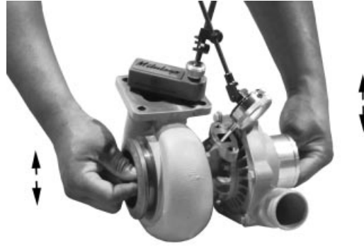
Radial Bearing Clearance Test
