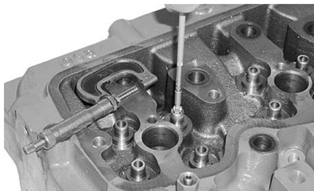
Valve Guide Wear
