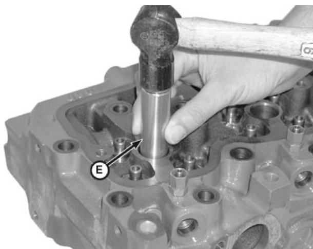
Fuel Injection Nozzle Sleeve Installation
