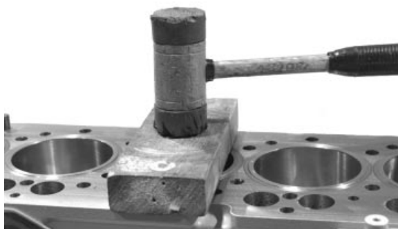
Install Cylinder Liner in Block
