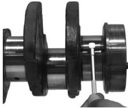
Measuring Main Thrust Journal Width
