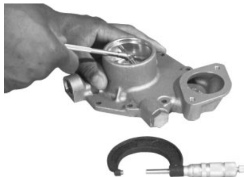
Coolant Pump Housing Weep Hole
