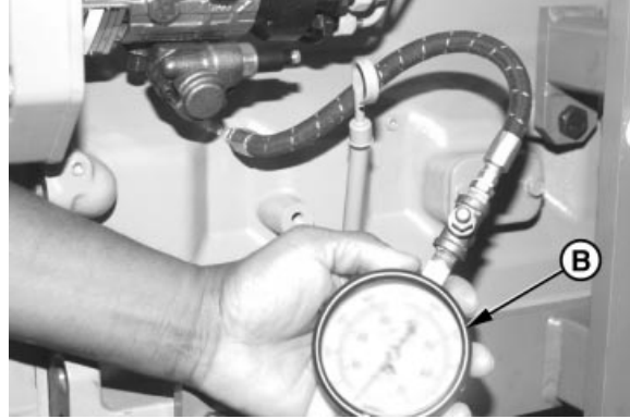
Pressure Gauge to Oil Gallery Port
