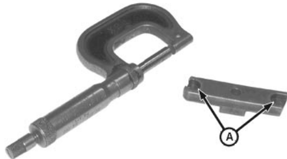
Inspect and Measure Bridges
