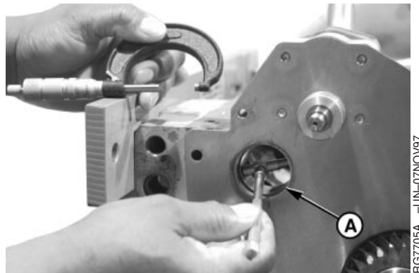
Measuring Balancer Shaft Bushing ID
