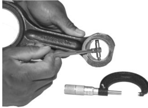
Measuring Connect Rod Pin Bore ID
