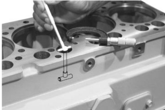
Measuring Camshaft Follower Bore
