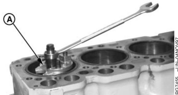
Using Ridge Reamer in Cylinder Bore
