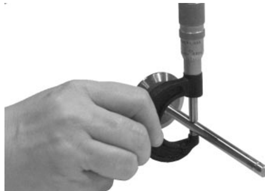
Valve Stem Measurement
