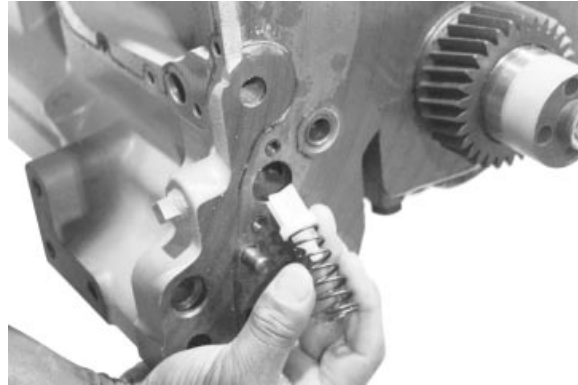
Oil Bypass Valve and Spring
