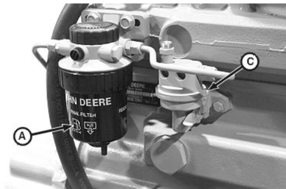
Fuel Filters and Supply Pump
