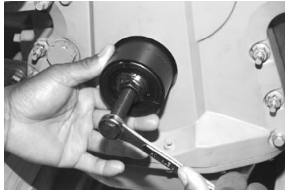
Front Wear Sleeve Removal Tool
