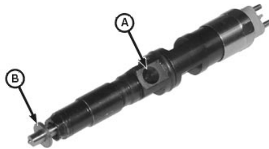
Fuel Injector Inlet Port
