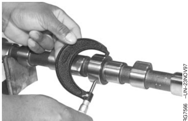
Measuring Camshaft Journal OD
