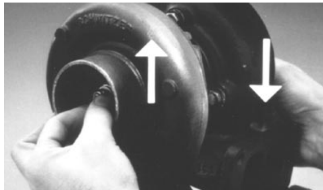
Checking for Contact of Compressor and Turbine Wheels
