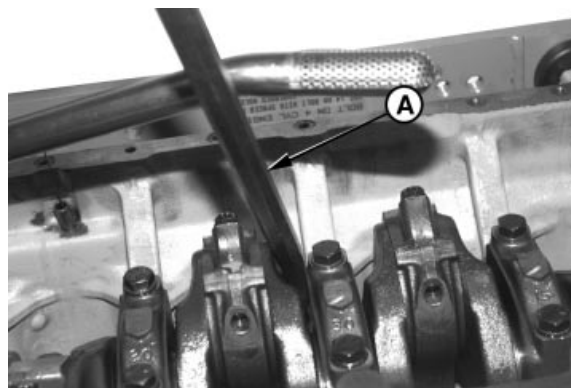
Prying Crankshaft Toward Rear of Engine
