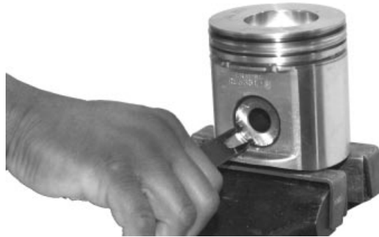
Piston Pin Snap Ring Removal
