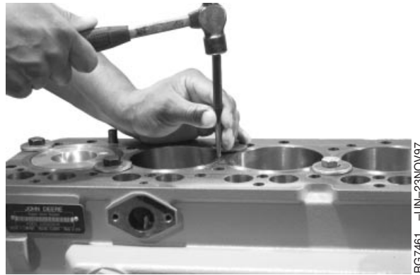
Marking Cylinder Liner Location/Position
