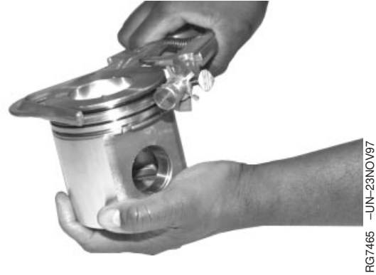
Cleaning Piston Ring Grooves
