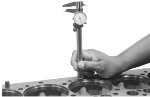
Measure Liner Flange Counterbore Depth
