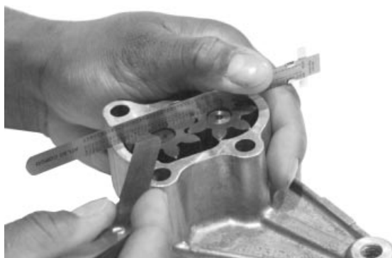
Checking Gear-to-Pump Cover Axial Clearance
