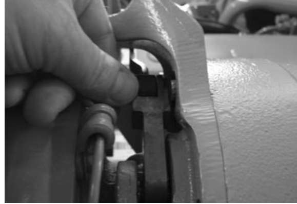
Check for Linkage Free Travel
