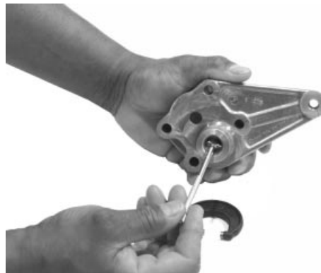
Measuring Bushing ID in Housing for Wear
