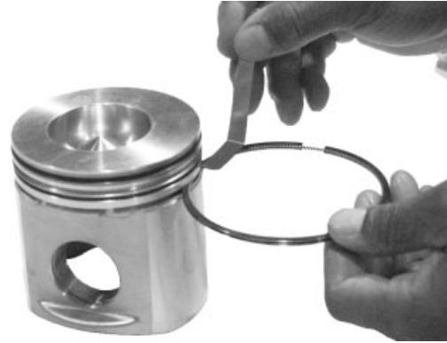
Piston Ring Groove Wear
