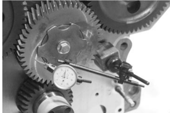
Measuring Idler Gear End Play
