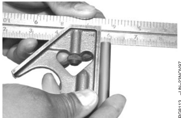
Push Rod End Crown Wear
