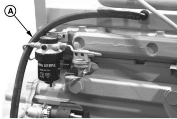
Ventilator Outlet Hose Inspection
