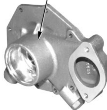
Inspect Coolant Pump Weep Hole
