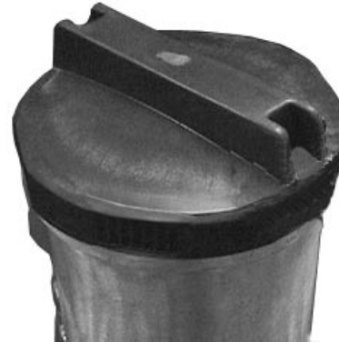
Remove Final Fuel Filter
